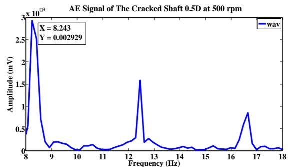
Fig. 7 AE signal of cracked shaft 0.5D at 500 rpm
