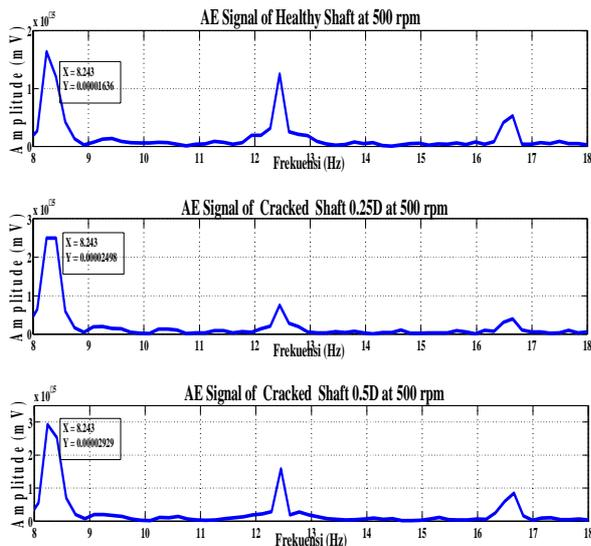
Fig. 10 AE signal of three test shaft at 500 rpm
