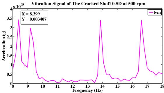
Fig. 9 Vibration signal of the cracked shaft 0.5D at 500 rpm
