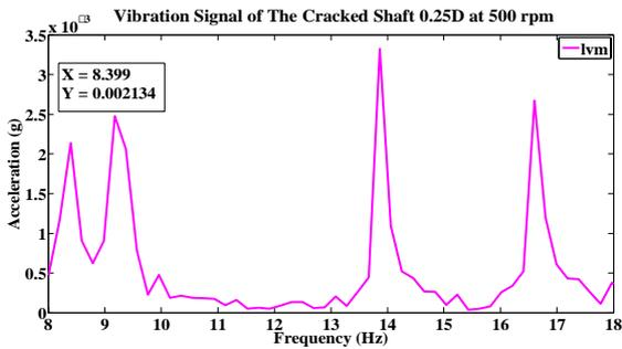
Fig. 8 Vibration signal of the cracked shaft 0.25D at 500 rpm
