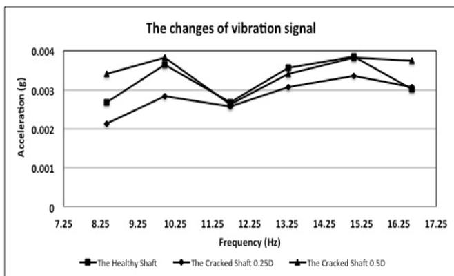
Fig. 5 The changes of vibration signal
