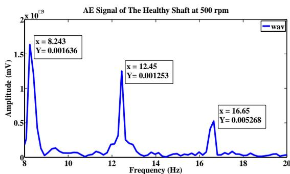
Fig. 2 AE signal of the healthy shaft at 500 rpm
