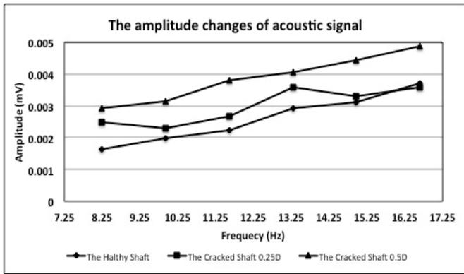
Fig. 4 Amplitude changes of AE signal at the healthy shaft
