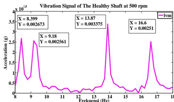
Fig. 3 Vibration signal of the healthy shaft at 500 rpm
