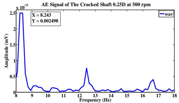
Fig. 6 AE signal of cracked shaft 0.25D at 500 rpm
