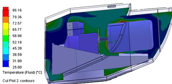
Fig. 7 Prediction of the ventilation system's working conditions in the Goldwind S 50/750 wind turbines installed in the Wind Farm Gibara II.
