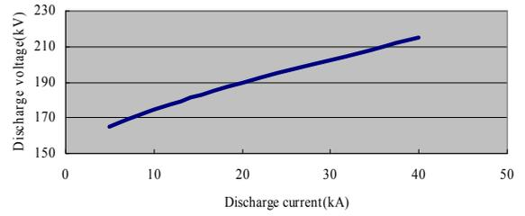
Fig. 4 V-I characteristic curve of line arrester
