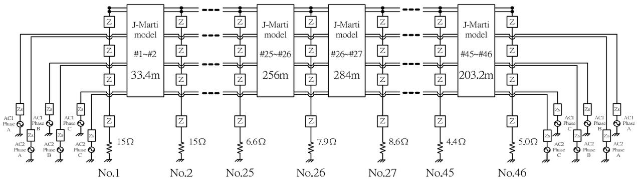
Fig. 5 Equivalent circuit for the selected transmission system
