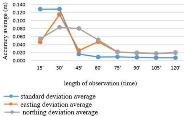
Fig 6. Standard, easting and northing deviation average
