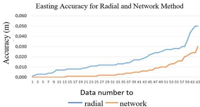
Fig 7 Comparison of easting accuracy between radial and network method
