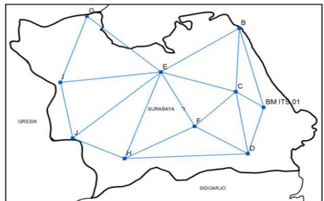
Fig 4. Network design of GCP measurements
