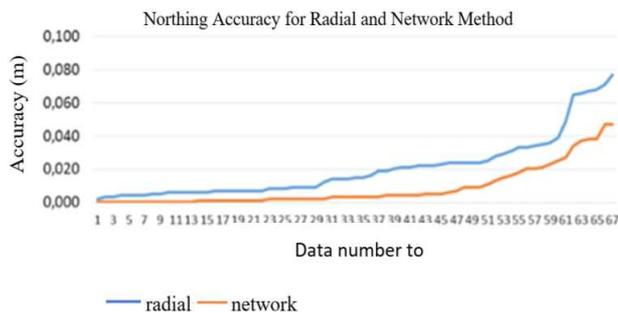
Fig 8. Comparison of northing accuracy between radial and network method
