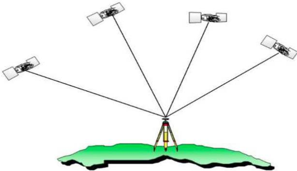
Fig 1. GNSS principle (resection with distance) [2]
