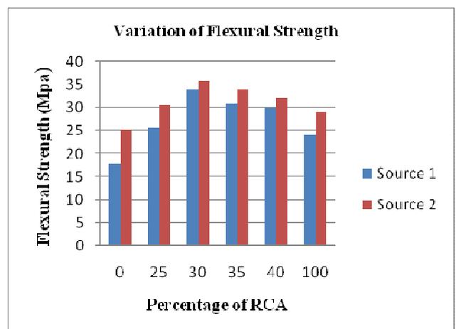
Fig. 4 Comparison of 28 days Flexural strength
