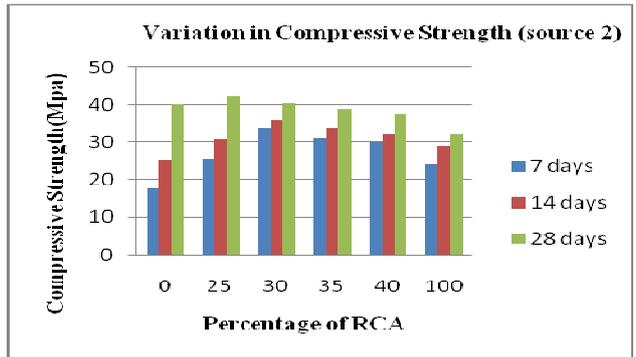
Fig. 2 Compressive Strength test results from source 2
