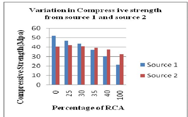
Fig. 3 Compressive strength results from source 1 and source 2
