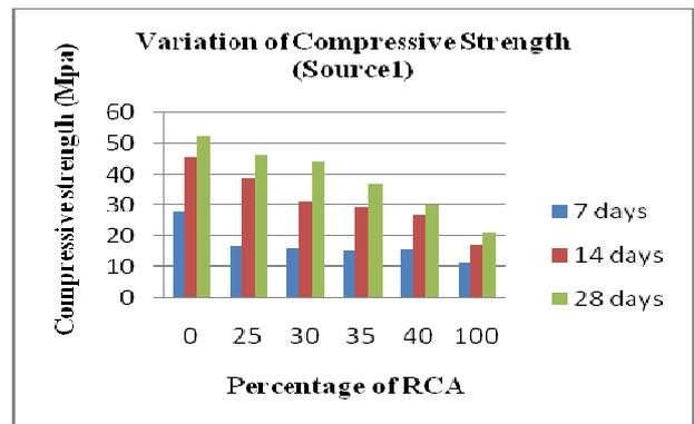
Fig. 1 Compressive Strength Test Results from Source 1
