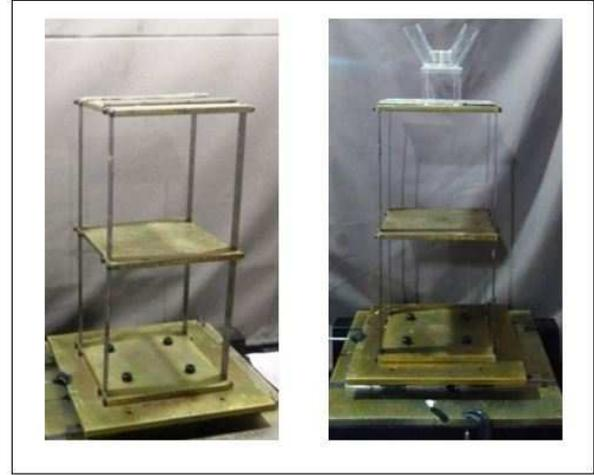
Fig. 4 (a) Structure without a TLCD (b) Structure equipped with a TLCD
