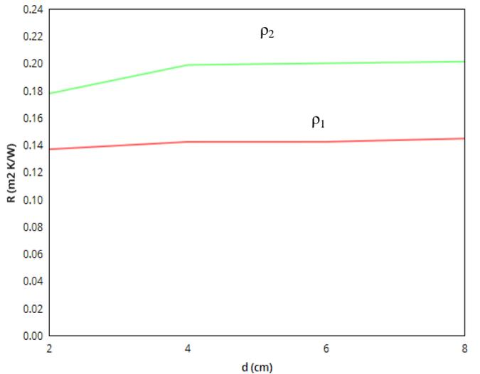
Fig. 6 Thermal resistance of sawdust with respect to thickness at  $\rho = 3.25 \text{ kg/m}^3$  and  $\rho = 64.875 \text{ kg/m}^3$
