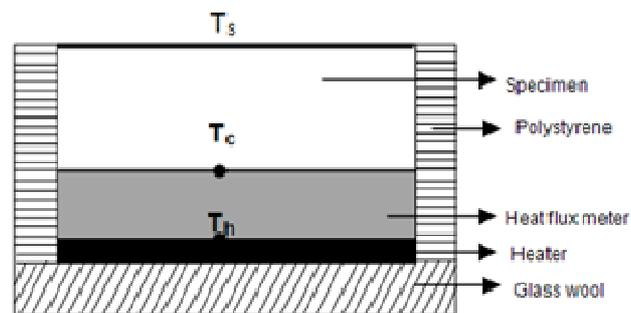
Fig. 1 Thermal measurement apparatus
