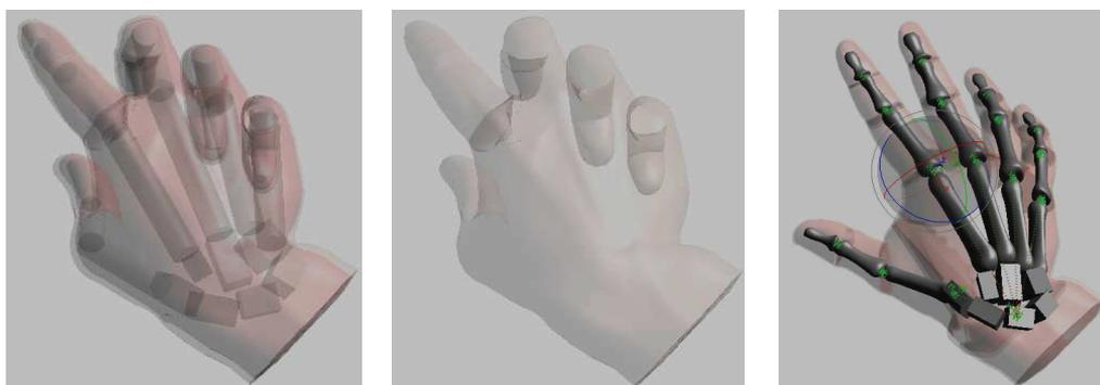
Fig. 2 (a). Homogeneous (H1), and (b) inhomogeneous (H2) hand models; (c) diagram of hand phantom modeling engine.
