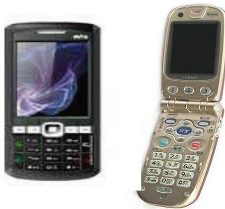
Fig. 1. Multiband phone used in this study: (a) a candy bar phone (b) a clam shell Phone
