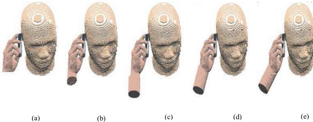
Fig. 4. The hand phantoms with different wrists: (a) no wrist, (b) 3cm long wrist, (c) 10cm long wrist (d) 10cm long 15 degrees tilted wrist, and (e) 10cm long 30 degrees tilted wrist
