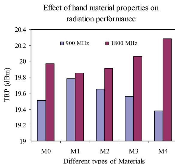
Fig. 3. Effect of hand material properties on radiation performance at 900 MHz and 1800 MHz
