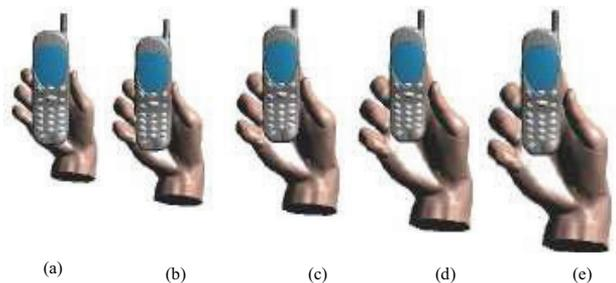
Fig. 6. The hand phantom different hand sizes for evaluating the influence of different mobile phone antenna performance: (a) 80 %, (b) 90 %, (c) 100 %, (d) 110 %, and (e) 120 % of the average hand size
