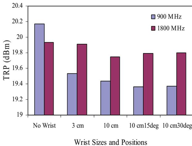
Fig. 5. Effect with different positions and different sizes on radiation performance at 900 MHz and 1800 MHz
