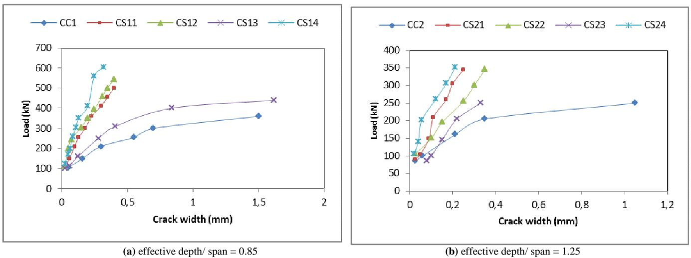
Fig. 8 Effect of strength configuration on development of crack width
