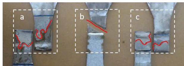
Fig. 6 Failure mechanism of A3M connection; (a) A3M50, (b) A3M75, (c) A3M100
