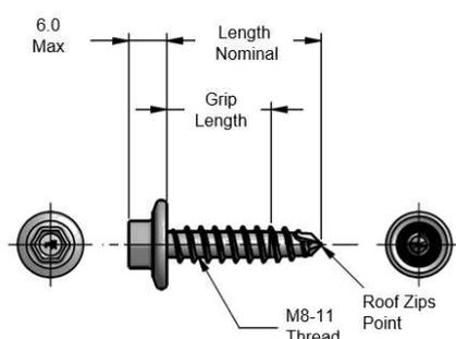
Fig. 4 Screw section detail
