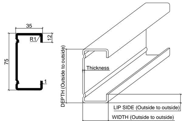
Fig. 1 Section geometry and dimension of CFS section (unit: mm)
