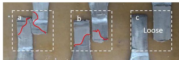
Fig. 7 Failure mechanism of ASK3M connection; (a) ASK50, (b) ASK75, (c) ASK100
