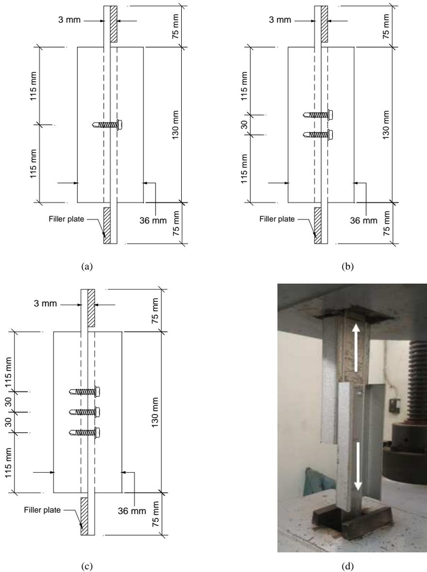
Fig. 3 Overall test set-up evaluating connection capacity
