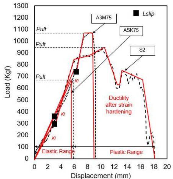
Fig. 9 Stress-strain diagram; S2-A3M75-ASK75
