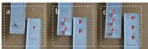
Fig. 5 Failure mechanism of Screw connection; (a) S1, (b) S2, (c) S3
