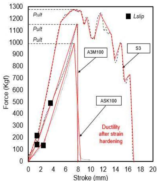
Fig. 10 Stress-strain diagram; S3-A3M100-ASK100
