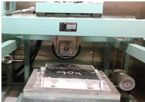
Fig. 2 Wheel tracking testing setup
