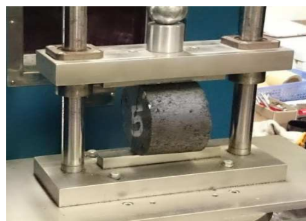
Fig. 1 IDT testing setup
