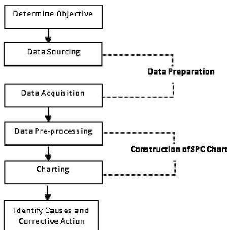
Fig. 1 Intrusion Detection System using Control Chart Method
