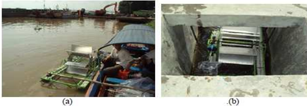
Figure 4: (a) Floating waterwheel on test on Musi River. (b) Floating waterwheel on test at sluice gate at Bangun Sari Village.
