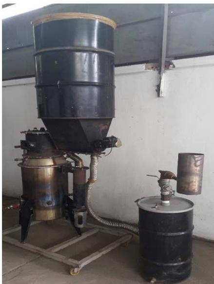
Fig. 1b. The downdraft gasifier
