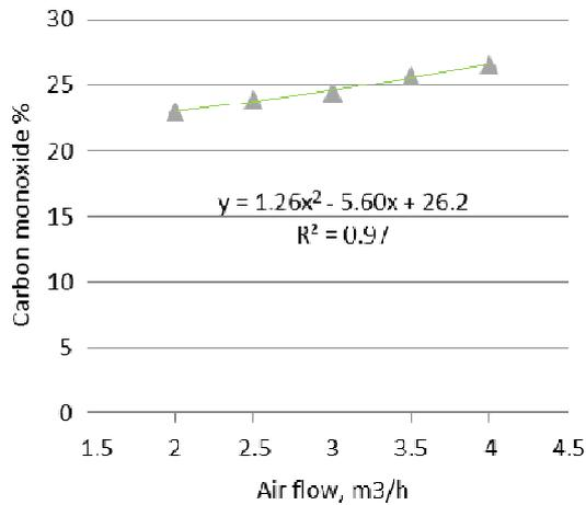
Fig. 6. Effect of air-flow on the Carbon monoxide
