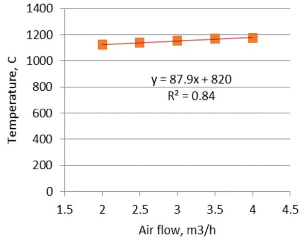
Fig. 4. Effect of air-flow on the syngas temperature
