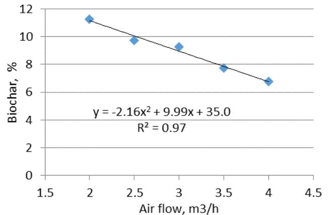
Fig. 9. Effect of air-flow on the biochar
