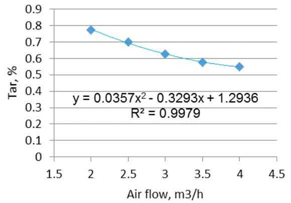
Fig. 8. Effect of air-flow on the Tar
