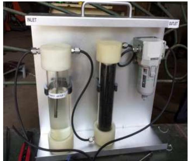
Fig. 2. The gasboard 3100P syngas analyzer
