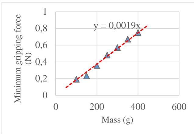
Fig. 6 Linear relationship between mass of the object and minimum gripping force
