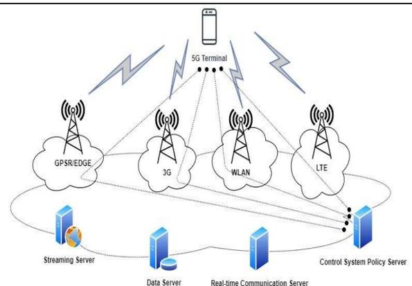
Fig.1 Functional architecture for 5G mobile networks [2].
