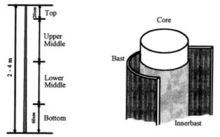
Fig. 2 Sampling positions and parts of kenaf stems [20], [21]
