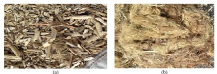
Fig. 3 (a) Kenaf core (b) Kenaf bast
