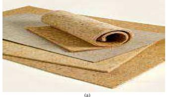
Fig. 6 (a) Natural fiber mat (b) Door inner panel
