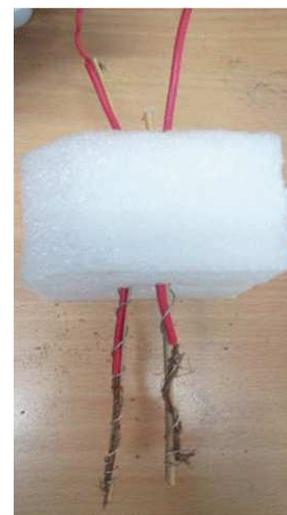
Fig. 3. Homemade Soil Moisture Sensor [39]
