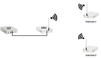
Fig. 4 Hardware configuration for CSMA/CA protocol
