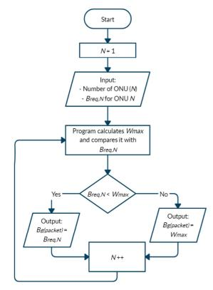
Fig. 6 Flowchart for DBA implemented in the proposed FiWi testbed
