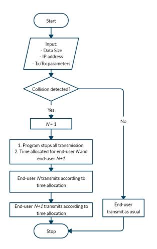
Fig. 5 Flowchart for the CSMA/CA algorithm
