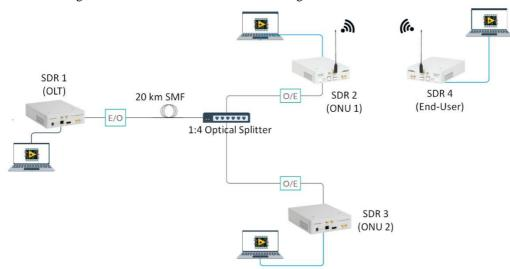
Fig. 1 Proposed FiWi testbed architecture
