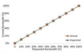
Fig. 9 Granted bandwidth vs requested bandwidth for DBA-Limited Scheduling
