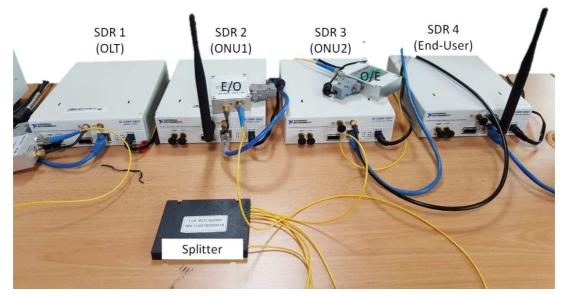
Fig. 2 SDR setup for the proposed FiWi testbed
