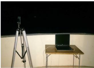
Fig. 3 Setting of the SQM device for ground measurements of sky brightness in the study area
