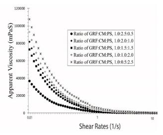
Fig 1. Apparent viscosity of ternary pastes of shear rate on the ratio of GRF, CM, and PS were 1.0:2.5:0.5, 1.0:2.0:1.0, 1.0:1.5:1.5, 1.0:1.0:2.0, and 1.0:0.5:2.5.
