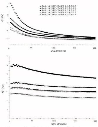
Fig 2. Storage modulus (G') (A) and loss modulus (G'') (B) of ternary paste (GRF-CM-PS paste) as a function of strain.
