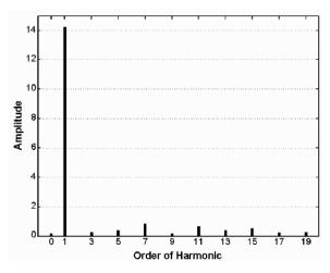
Fig. 8 Odd Harmonics after Input-Current Shaping
