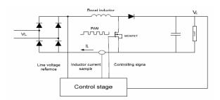
Fig.1S<sup>4</sup>ICS Circuit Utilizing Boost DC-DC Switching Converter
