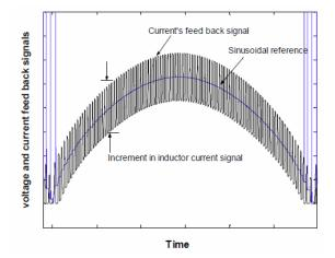
Fig.2 Simulation Shows How the Boost Inductors Ripples Follow the Sinusoidal Reference
