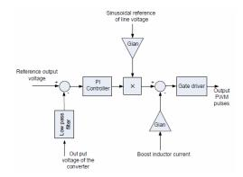
Fig. 3 PWM Controller with two Feed Back Loops
