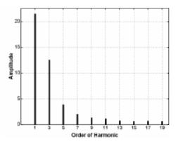
Fig. 7 Significant Odd Harmonics Plot Prior to the Input-Current Shaping TABLE II SIGNIFICANT ODD HARMONICS LEVELS PRIOR TO THE INPUTCURRENT SHAPING
