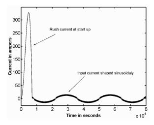
Fig. 4 Shows the Input Line Current after Input-Current Shaping
