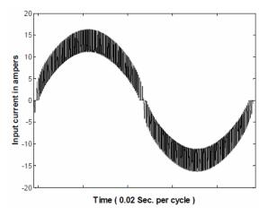
Fig. 5 Inductor Current Made of Charging and Discharging Phases
