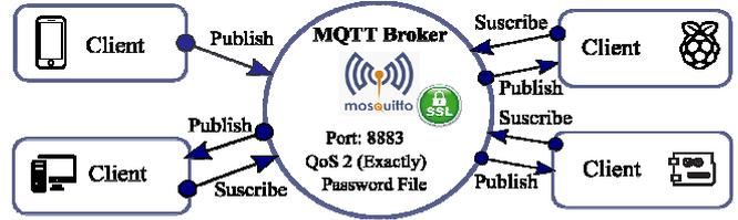
Fig 7. Real-time notification system.
