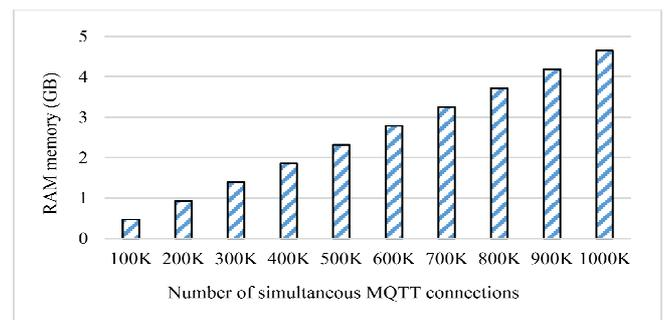
Fig 12. Memory required for MQTT connections
