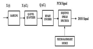
Fig.2: DSSS encoding scheme for voice signal.
