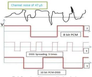
Fig.8: Comparison of bits corrupted by channel noise.
