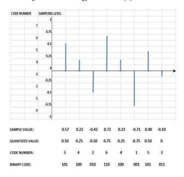
Fig. 6: Encrypted samples of 3 bit encoding scheme.
