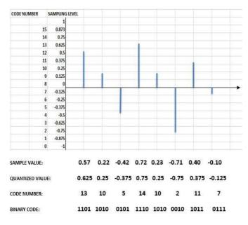
Fig. 7: Encrypted samples of 4 bit encoding scheme.
