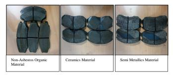
Fig. 2: Types of Brake Pads Used in the Study
