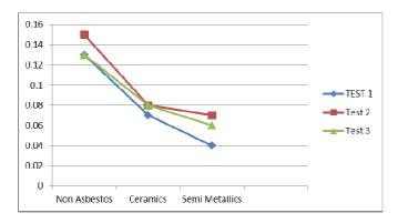
Fig. 5: Graph of Test Results for 3 types of Brake Pads (Thickness Loss)
