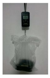
Fig. 4: Weighing Equipment used for weighing the brake pads
