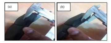
Fig. 3: Vernier caliper is used to measure the brake pads wear (a) measure the thickness of brake pad with backing plate (b) measure thickness of backing plate
