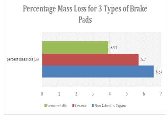
Fig. 6: Graph of Percentage Mass Loss for 3 types of Brake Pads
