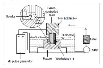
Fig. 1 Schematic of an EDM die sink process
