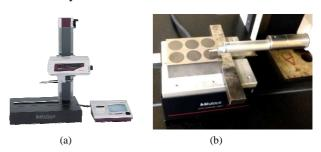
Fig. 6 (a) Mitutoyo surface roughness tester; (b) actual measurement of machined profiles on Ti6Al4V specimen
