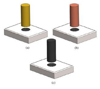
Fig. 2 EDM Process on titanium block using (a) copper electrode, (b) brass electrode, (c) graphite electrode
