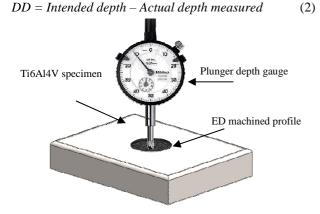
Fig. 7 Depth measurement of the ED machined Profile
