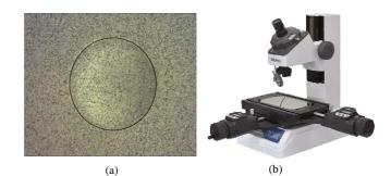
Fig. 5 (a) Actual impression on the Ti6Al4V specimen; (b) Mitutoyo toolmaker's microscope
