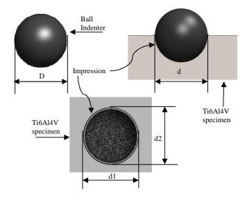
Fig. 4 Brinnel hardness measurement procedure
