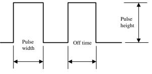
Fig. 3 Current pulse waveform
