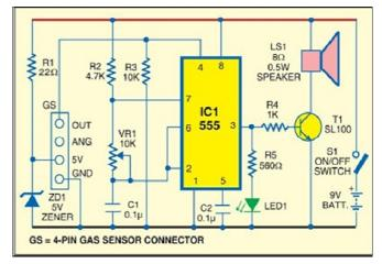
Fig. 2 "Circuit Diagram of Exhaust Leak Detector"
