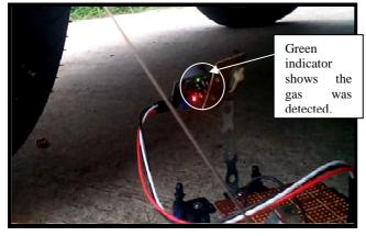
Fig. 6 Sensor Indicator (Green Light) Detect the Leakage from Exhaust Pipe
