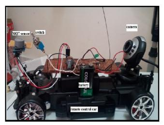
Fig. 5 Final Installation of Exhaust Leak Detector Device
