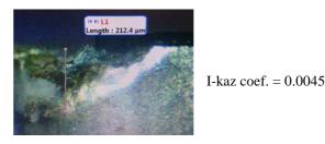
Fig. 9 Wear status and I-kaz coef. Values for Run 6 at DOC 0.4 mm
