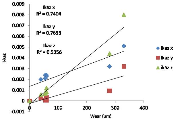
Fig. 4 Correlation between the I-kaz<sup>TM</sup> multilevel coefficient and flank wear at 0.4 mm depth of cut
