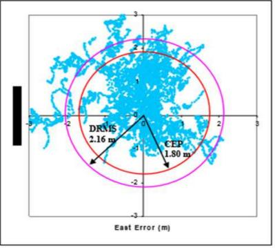
Fig. 1. The vessel position in circular error probability [15]
