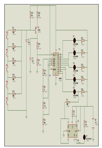
Fig. 8 Water level indicator schematic circuit
