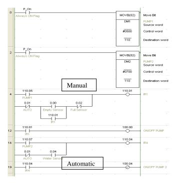
Fig. 18 Ladder diagram for connecting with IGSS
