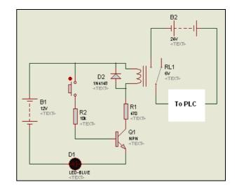
Fig. 5 Interface circuit for relay
