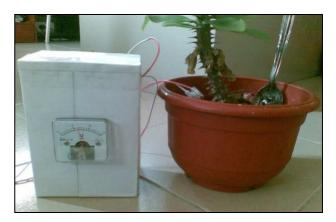
Fig. 11 Water detector unit
