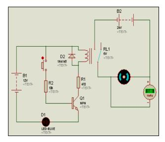
Fig.12 PLC interface schematic circuit
