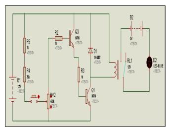
Fig. 10 Water sensor detector circuit
