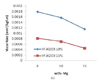
Fig.1 Effect of Mg on mechanical properties of Al6061/Al\_2O\_3 metal matrix composites produced by double blade stir casting. a) Tensile strength, b) Hardness, c) Wear rate.
