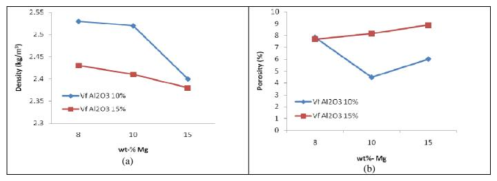
Fig. 2 Effect of Mg on density (a) and porosity (b) of Al6061/Al<sub>2</sub>O<sub>3</sub> metal matrix composites produced by double blade stir casting.
