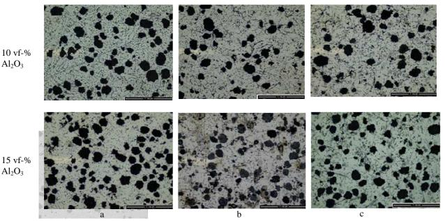
Fig. 3 Distribution of Al<sub>2</sub>O<sub>3</sub> particles with different Mg and Al<sub>2</sub>O<sub>3</sub> content in an Al 6061 matrix on metal matrix composites produced by double blade stir casting. a) 8wt-% Mg, b) 10 wt-% Mg and c) 15wt-% Mg
