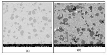
Fig.5 SEM micrograph of Al/Al<sub>2</sub>O<sub>3</sub> composite with 10 vf-% Al<sub>2</sub>O<sub>3</sub>-10 wt-% Mg (a) and (b) microstructure of Al/Al<sub>2</sub>O<sub>3</sub> composite with 15 vf-% Al<sub>2</sub>O<sub>3</sub>-15 wt% Mg
