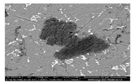
Fig. 6 SEM micrograph of Al/Al<sub>2</sub>O<sub>3</sub> composite with 10 vf-% Al<sub>2</sub>O<sub>3</sub>-10 wt-% Mg link to EDS to identify phase presence in composite
