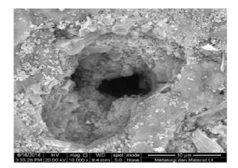
Fig.7 Fracture surface of Al/Al\_2O\_3 composites taken from the tensile sample with 15wt-% Mg and 15 vf-% Al\_2O\_3\_
