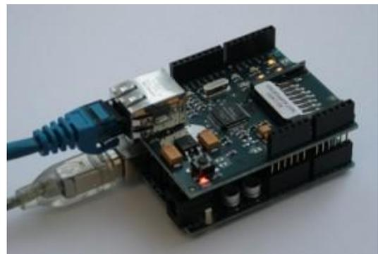
Fig.5 Arduino Duemilanove and Ethernet Shield
