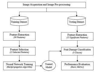
Fig. 3 The system architecture of jackfruit fruit damage recognizer
