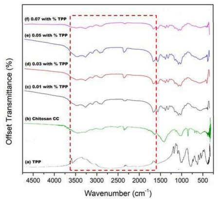
Fig 2. FT-IR Spectrum of the prepared Coconut Crab Chitosan (Chitosan CC) at various TPP concentration. a) TPP, b) Chitosan CC, c) 0.01 with % TPP, d) 0.03 with % TPP, e) 0.05 with % TPP, f) 0.07 with % TPP.
