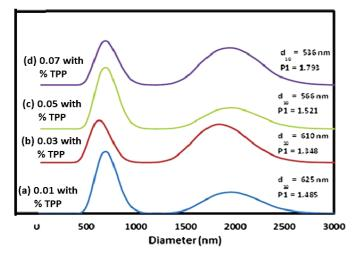
Fig 3. A). Image of Chitosan CC with TPP suspension. **B**). PSA of the preperied Coconut Crab Chitosan (Chitosan CC) at various TPP concentration. **a**) 0.01 with % TPP, **b**) 0.03 with % TPP, **c**) 0.05 with % TPP, **d**) 0.07 with % TPP.
