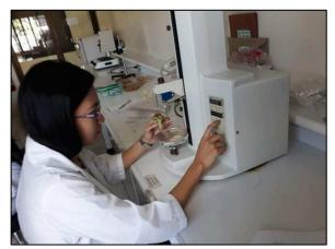
Fig. 2 Shimadzu Table Top Type Tester-EZTest Series
