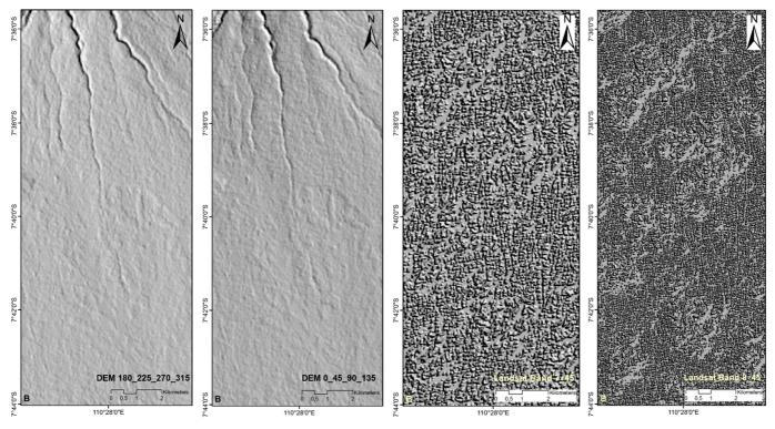
Fig. 3. Hill-shaded image from four directions with lighting from various azimuth angle of  $180^{\circ}-225^{\circ}-270^{\circ}-315^{\circ}$  for positive relief features and  $0^{\circ}-45^{\circ}-90^{\circ}-135^{\circ}$  for negative relief features. Landsat 8 band 7 (30 m resolution) and 8 (15 m resolution) with the  $45^{\circ}$  the light source azimuth angles.
