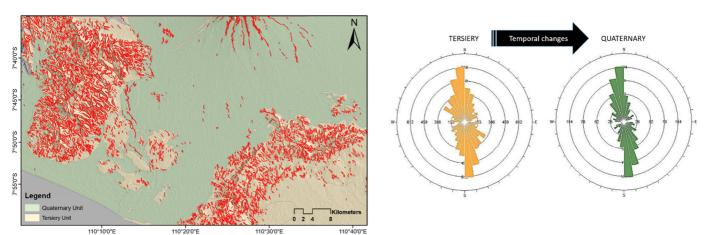
Fig. 7. Lineaments spatial distribution using DEM 30 m through the geologic units with lineaments strike and frequency direction over the rocks unit.
