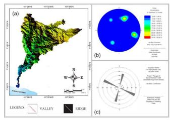
Fig. 9 (a) The geological structure analyzes of the study area in the form of lineament of valley and ridge on SRTM-DEM image with the general direction of NW-SE and NE-SW, (b and c) joints analysis use DIP program with the general direction of NW-SE and NE-SW.
