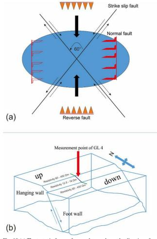
Fig. 10 (a) The tectonic frame of research area shows the direction of main force azimuth relatively from South to North on Quarternary period. (b) The illustration of normal fault in GL 4 with azimuth direction of North-South.
