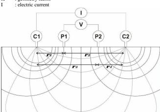
Fig. 4 Electrode Schlumberger configuration geoelectric method
