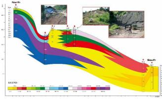
Fig. 7 The lithology cross section, of geoelectric measurement, GL1-GL7 trajectory with height of 195 to 925 meters a.s.l, depth of up to 120 meters and resistivity values of 6 to 450  $\Omega$  meters in the Cilaki drainage basin
