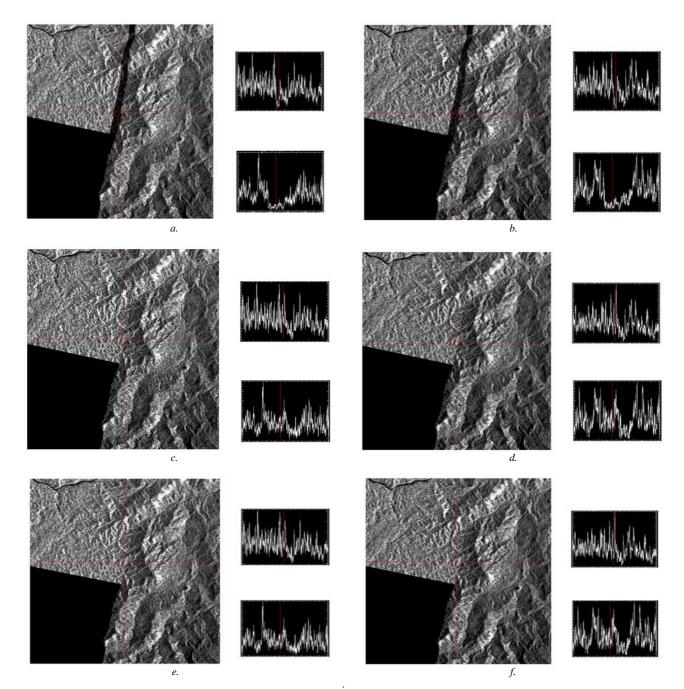
Fig. 5 Mosaic products, horizontal and vertical profile; a. VH, b. VV GRD raw data, c. VH, d. VV S-1 Remove GRD Border Noise results, e. VH, f. VV Random Noise Removal results.
