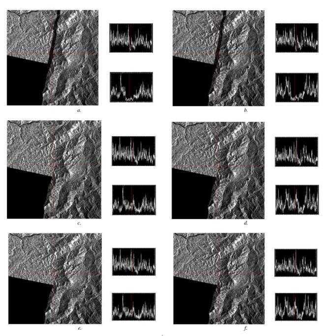
Fig. 5 Mosaic products, horizontal and vertical profile; a. VH, b. VV GRD raw data, c. VH, d. VV S-1 Remove GRD Border Noise results, e. VH, f. VV Random Noise Removal results.
