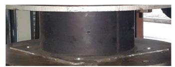
Fig. 16 Vertical-test sample A1 at the vertical displacement of 28 mm
