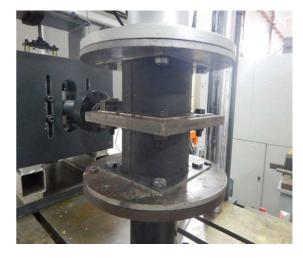
Fig. 9 Horizontal test setup on MTS 322 servo-hydraulic machine
