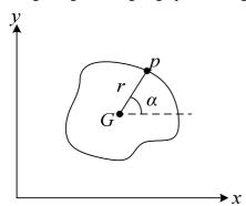
Fig. 1 Illustration of Centroid Contour Distance
