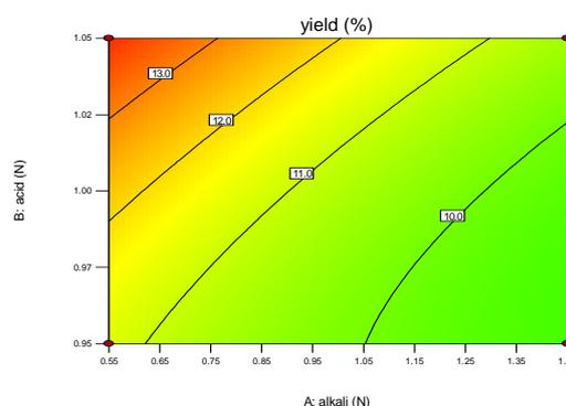
Fig. 2. The response surface plots of gelatin yield of black spotted oceanic triggerfish waste
