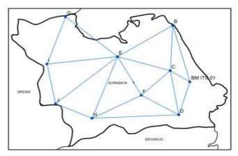
Fig 4. Network design of GCP measurements
