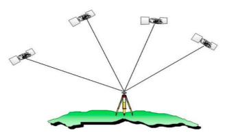
Fig 1. GNSS principle (resection with distance) [2]
