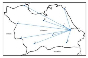
Fig 3. Baseline design of GCPs measurements
