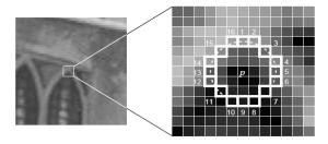
Fig .2 12 point segment test corner detection in an image patch . The highlighted squares are the pixels used in the corner detection . The pixel at p is the centre of a candidate corner . The arc is indicated by the dashed line passes through 12 contiguous pixels which are brighter than p by more than the threshold .
