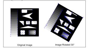
Fig .1 Rotational instability of Harris operator due to anisotropic response
