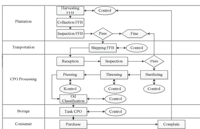
Fig. 4 Production process flow of CPO
