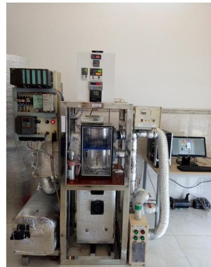
Fig. 11 The heat – pump dryer with ultrasound
