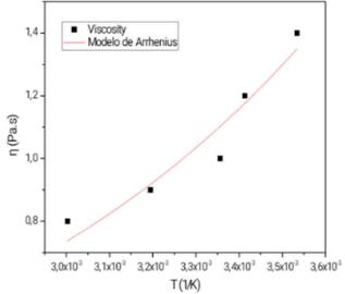
Fig. 2 Variation of the values of  $\eta$  obtained at 17 s-1 as a function of temperature and adjustment to the Arrhenius equation.
