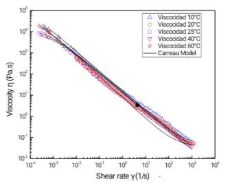
Fig. 1 Viscous flow curves of C. Melo pulp at different temperatures (10, 20, 25, 40, 60 °C) adjusted to the Carreau-Yasuda model.
