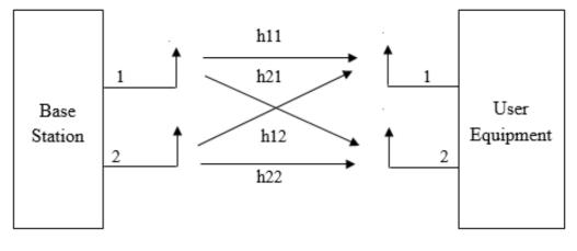
Fig. 1 Basic representation of Alamouti space-time block encoder
