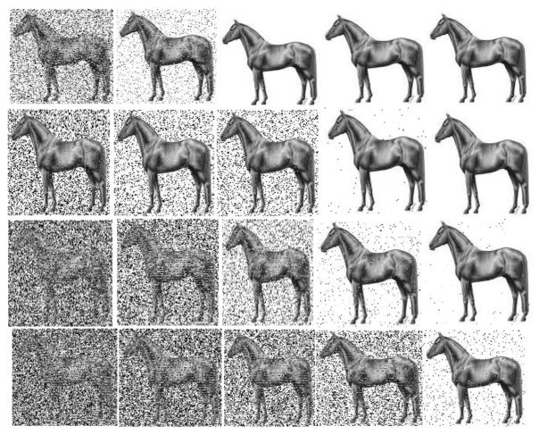
Fig.7 Image received for M-PSK using Alamouti Space-Time Coding with 2 receiver antenna at different SNR values (Column-wise: 0dB, 10dB, 20dB, 30dB and 40dB) for diverse modulation levels (Row-wise: 8-PSK, 16-PSK, 32-PSK and 64-PSK)
