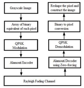
Fig. 3 Flowchart of image transmission using MIMO-Alamouti coding
