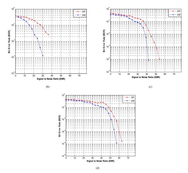
Fig. 4: SNR vs. BER plots for M-PSK using Alamouti MIMO channel model with diverse antenna configurations over Rayleigh channel a) 8-PSK b) 16-PSK c) 32-PSK d) 64-PSK
