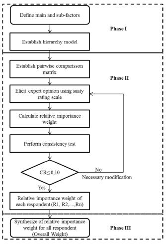
Fig. 1 Flowchart of the AHP method
